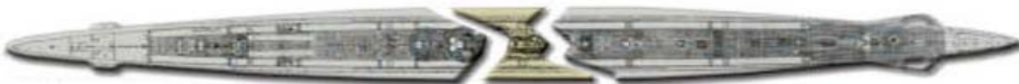
Top view: U-864 was hit by a torpedo in the middle section, and was split in three parts
